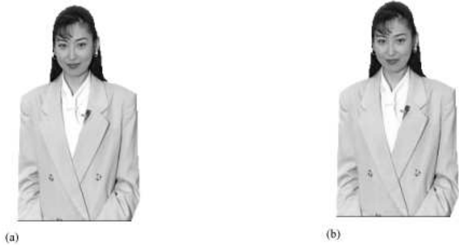
Figure 10: Frame 1 of the Weather video sequence: (a) the original image and (b) the image coded by the proposed BBS algorithm with the threshold value T = 4 (bit rate = 1 bpp and PSNR= 31.8 dB).
