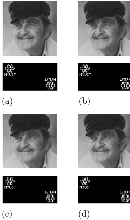
Figure 9: Simulation result of the proposed method. Upper row shows the superposed images I(\xi, \eta) and lower row shows the reconstructed images g_r(x, y) . (a) \alpha = 1/1 , \sigma_I = 0.37 ; (b) \alpha = 1/5 , \sigma_I = 0.51 ; (c) \alpha = 1/10 , \sigma_I = 1.43 ; (d) \alpha = 1/50 , \sigma_I = 7.19 .
